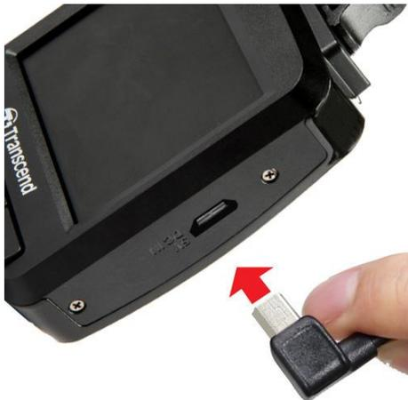
2. Connect the Type-A connector to the dual USB car charger, and plug the car charger into your car power outlet.
