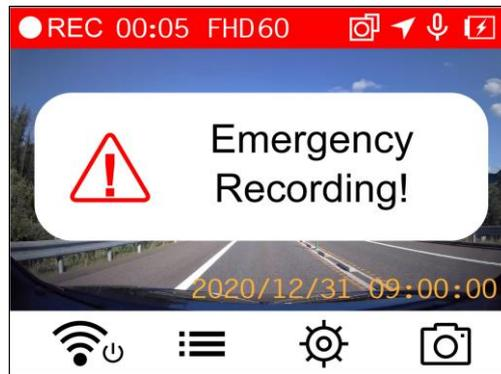
**G-Sensor Emergency Recording:** During video recording, the DrivePro will automatically activate Emergency Recording mode when detecting a collision.
