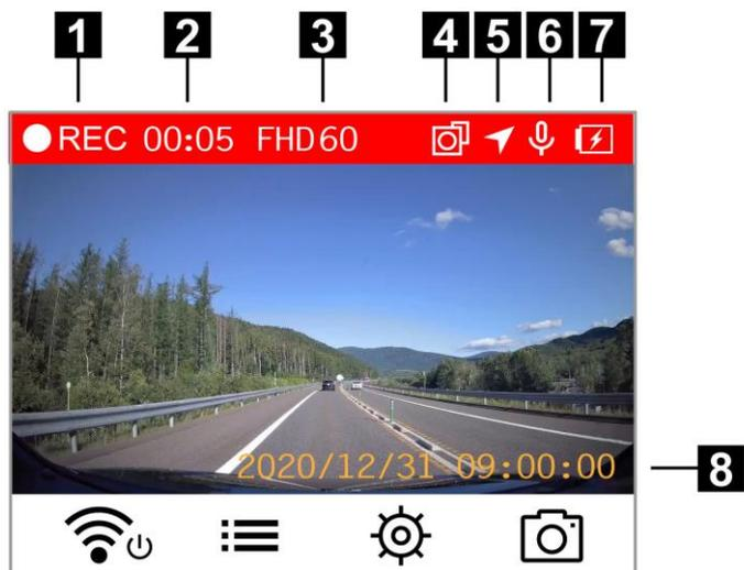
After the car engine is switched on, the DrivePro will automatically turn on and start recording. By default, one video file is saved for every 1 minute of recording. To adjust the recording length, please refer to the Settings section in this manual.
