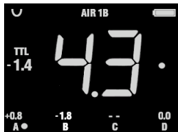
Example of Display [9] settings in TTL mode operation
